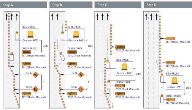
Figure 5.5 Removal of Two Right or Two Left Lane Closure (Freeway with Shoulders)
